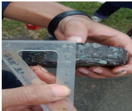
Gambar 3. Hasil core drill jalan kampus Polinela
